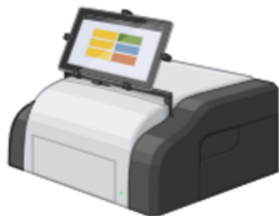
Measure dye bath exhaustion at 615 nm
