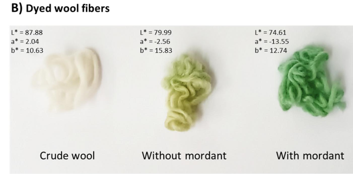
Fig.1 Chlorophyll uptake (%) of the wool fibers with and without CuSO_4 as mordant (A) and the visual aspect of the dyed wools (B) after one dyeing cycle (i.e., 60 min at 50 °C). The L^* , a^* and b^* colorimetric parameters of each type of wool fiber are presented at their left superior side. Undyed mordanted fibers presented L^* , a^* and b^* values of 73.71, 17.78 and 6.18, respectively.
